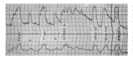
**Figure 2.** Parallel recordings of acoustic input impedance measured in the ear canal (top trace) and speech sound pressure level (lower) show that the two track each other almost instantaneously, demonstrating that the middle ear muscles contract and release very quickly (in less than a small fraction of a second). Time scale: 1 square is approximately 0.1 second. Reproduced from (19) with permission
